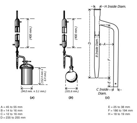
FIG. 1 Apparatus for Determining Water Content
